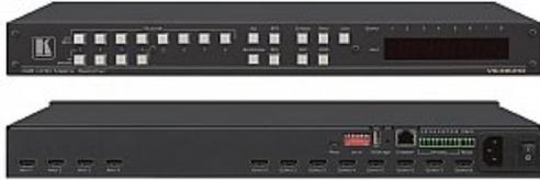
VS-48UHD is a high-quality 4x8 matrix switcher for 4K@60Hz (4:2:0) HDMI signals and embedded audio. It reclocks and equalizes the signals and can route any one of four HDMI, HDCP-compliant sources (selectable) to any or all outputs simultaneously. VS-48UHD offers a flexible audio scheme where any HDMI digital audio input can be routed to any HDMI digital audio output in addition to ARC support to produce an equivalent 12x10 audio matrix
